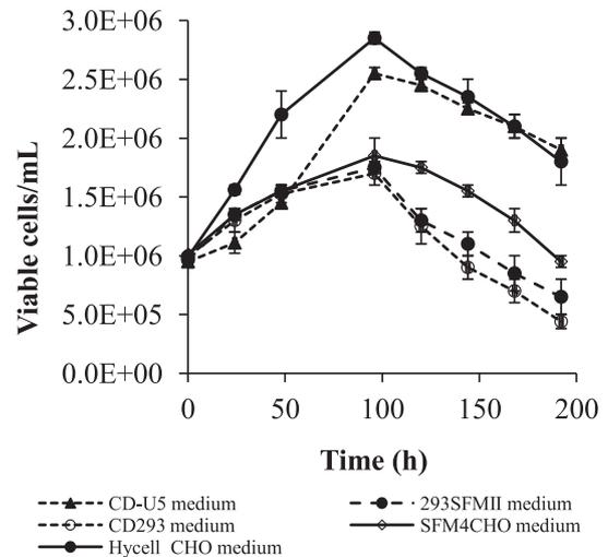
**Fig. 6.** Growth profile of VeroS grown in shake flasks in IPT-AFM and 5 commercial serum free/chemically defined media. The error bars represent the standard deviation of three experiments.
